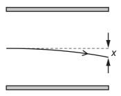
The vertical deflection *x* is measured at the right-hand edge of the plates.
