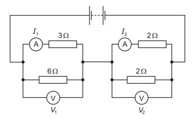
The readings on the meters are  $I_1$ ,  $I_2$ ,  $V_1$  and  $V_2$ , as labelled on the diagram.
